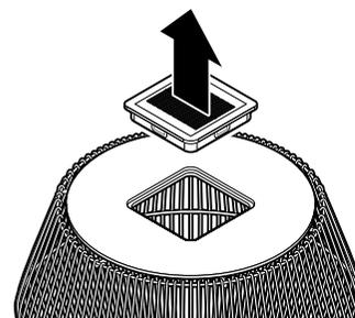
▷ To remove the module, reach into the base frame **from below** and push the solar module upwards to remove it.
