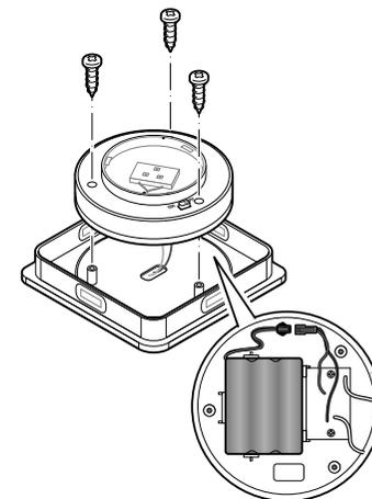
3. Use a Phillips screwdriver to loosen the screws on the bottom of the solar module and carefully remove the cover.
