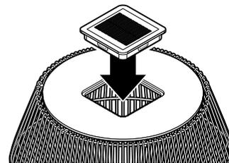
▷ To insert the solar module, insert it into the tabletop **from above**.
